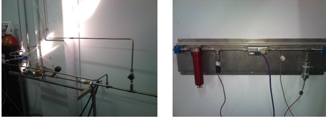
Figure 2 Syngas feeding system
