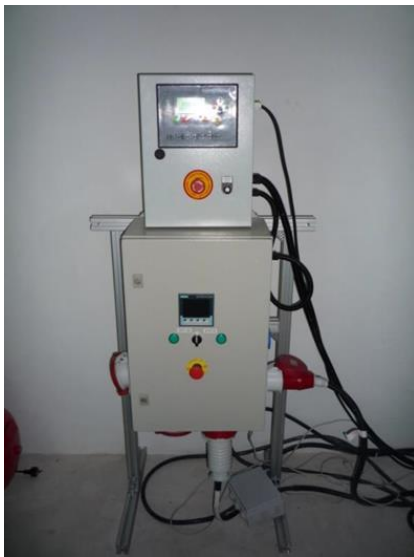
Figure 4 Power measurement and resistive load
