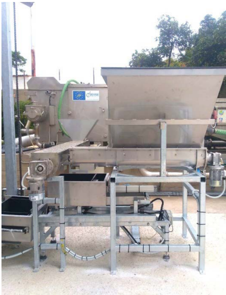
Feeding system of the dryer (screw conveyors and silos, weighing/dosing container, elevator)
