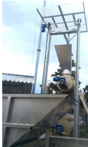
Feeding system of the dryer (screw conveyors and silos, weighing/dosing container, elevator)
